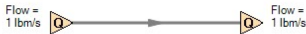
Figure 1: Model with two assigned flows. This model does not have a unique solution
