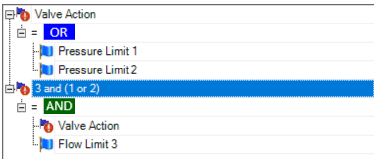
Figure 5: A Multi-Condition Event containing another Multi-Condition Event (trigger if Limit 3 AND (Limit 1 OR Limit 2))
