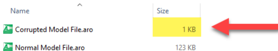
Figure 2: Very low file sizes can be an indication of model file corruption
