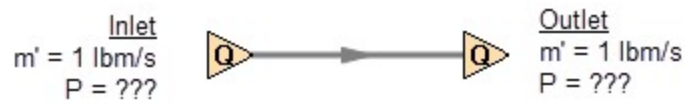
Figure 1: Model with two assigned flows. This model does not have a unique solution.
