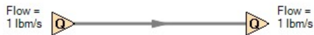
Figure 1: Model with two assigned flows. This model does not have a unique solution
