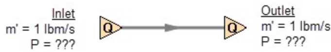
Figure 1: Model with two assigned flows. This model does not have a unique solution.
