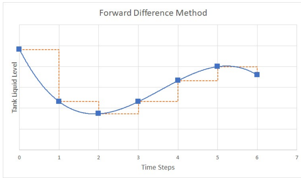
Figure 1: Forward difference method for time calculation assumes liquid level stays constant during each time step, allowing a direct calculation for each time
