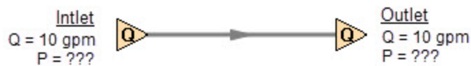
Figure 1: Model with two assigned flows. This model does not have a unique solution.
