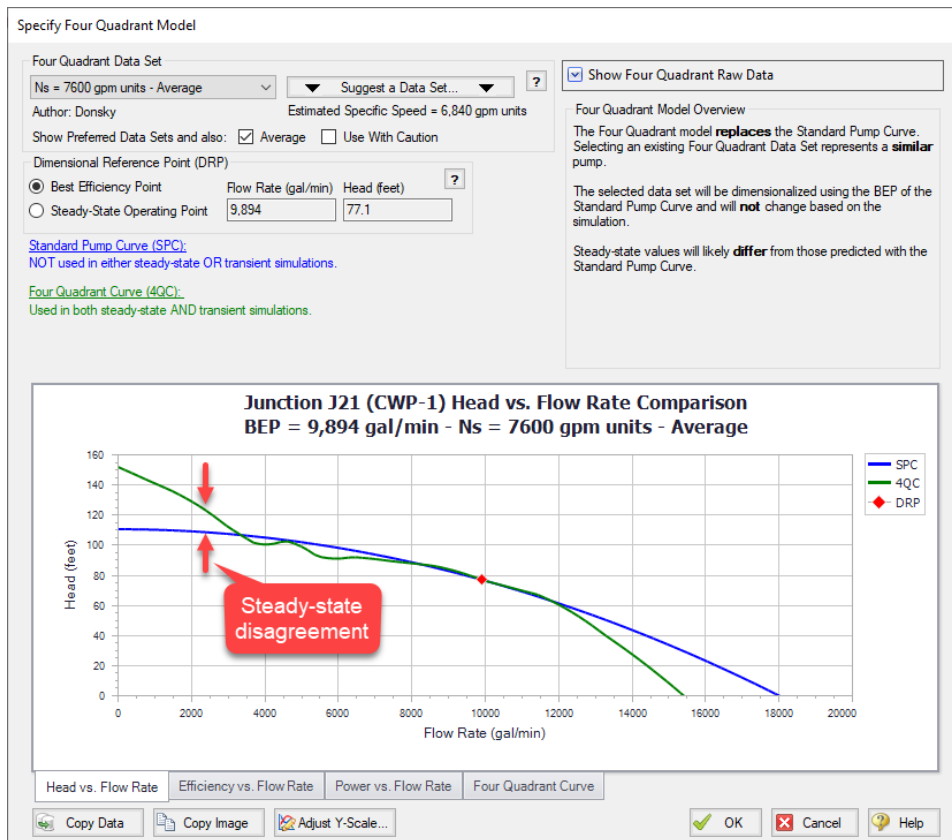
Figure 2: Using Best Efficiency Point as the DRP. The Four Quadrant Curve is static and disagrees in some areas with the Standard Pump Curve. However, the curve matches reasonably, especially near BEP.
