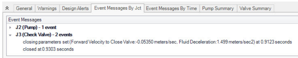
Figure 10: The event message tab provides additional information on the fluid deceleration calculations at the check valve. The non-dimensional case is shown here.
