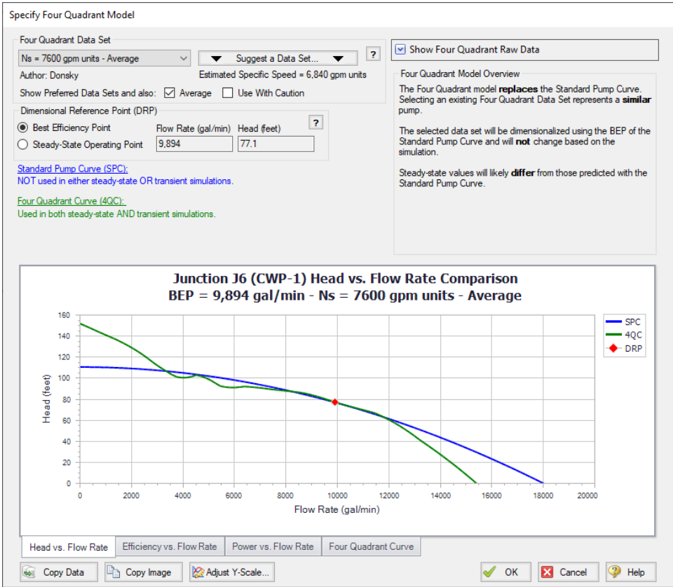
Figure 6: The Define Four Quadrant Model window can be used to select and view options for the dimensionalized four quadrant data set
