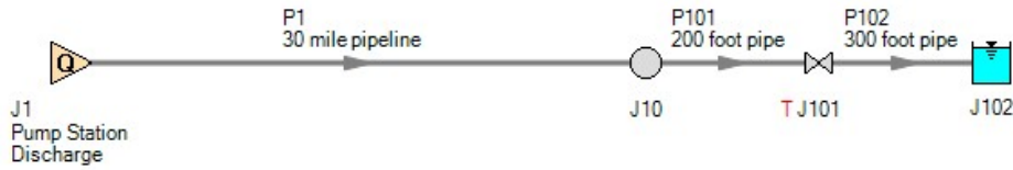
Figure 1: Example application of infinite pipe
