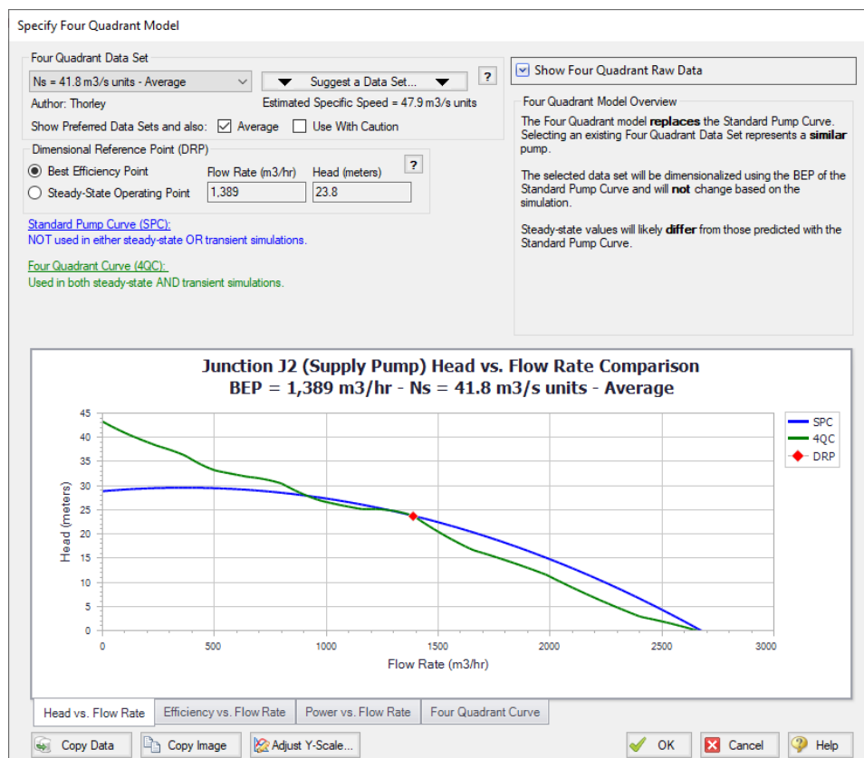
Figure 7: Specify Four Quadrant window showing the Head vs Flow data for the Ns = 41.8 data set dimensionalized using the BEP
