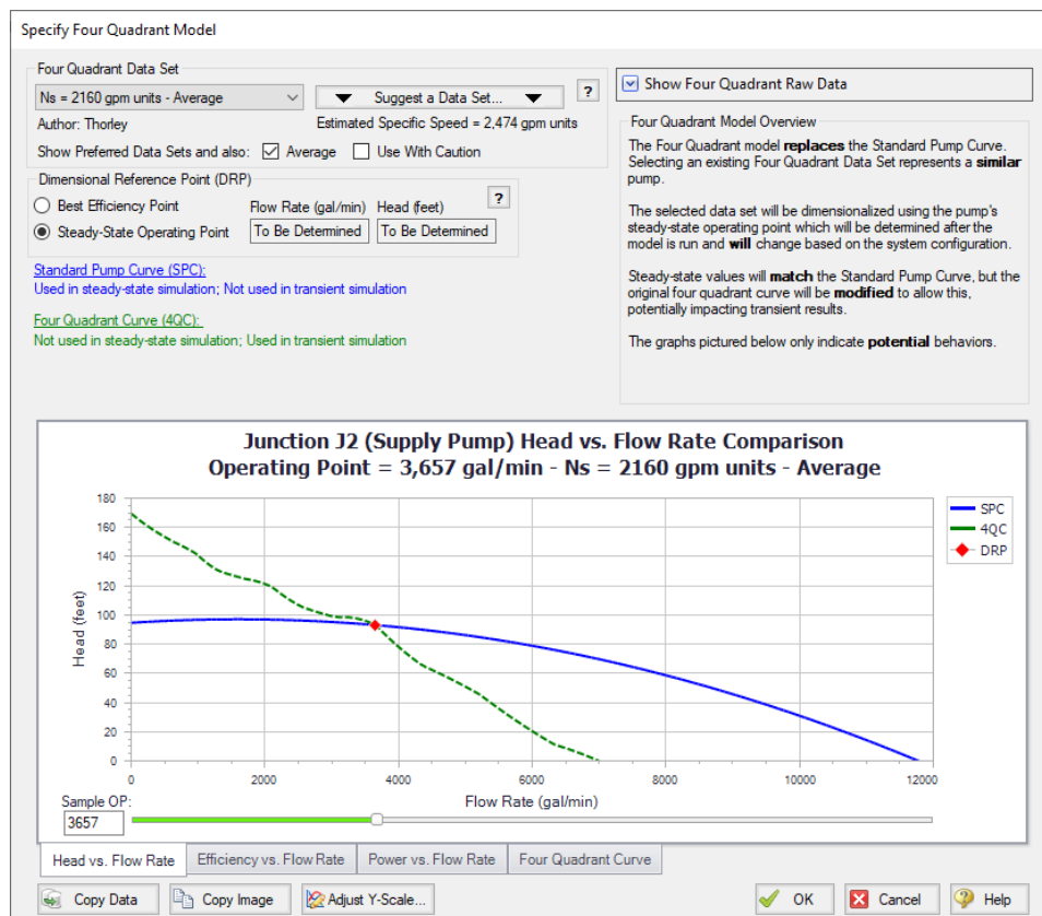
Figure 9: Specify Four Quadrant window showing the Head vs Flow data for the N_s = 2,160 data set dimensionalized using the SSOP, which is 3,656 gal/min for this scenario
