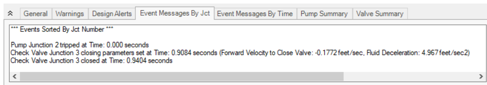
Figure 10: The Event Messages tab provides additional information on the fluid deceleration calculations at the check valve. The non-dimensional case is shown here
