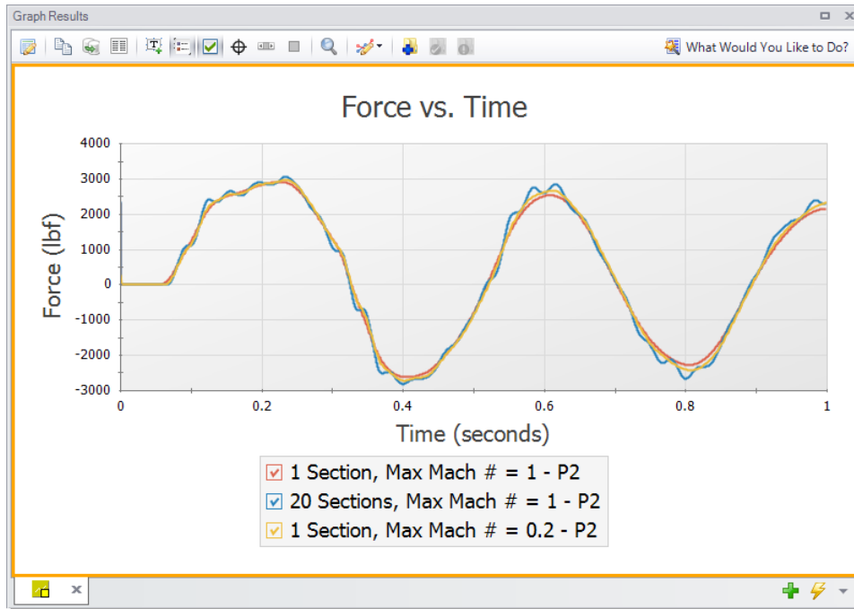
Figure 20: Effect of Maximum Pipe Mach Number During Transient on High Pressure Steam - Forces model. All runs use the AFT Standard fluid library.
