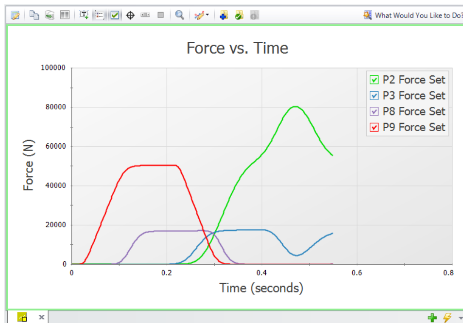
Figure 2: Force Results for AFT Standard, 10 Minimum Sections, Standard Maximum Mach Number in Pipe
