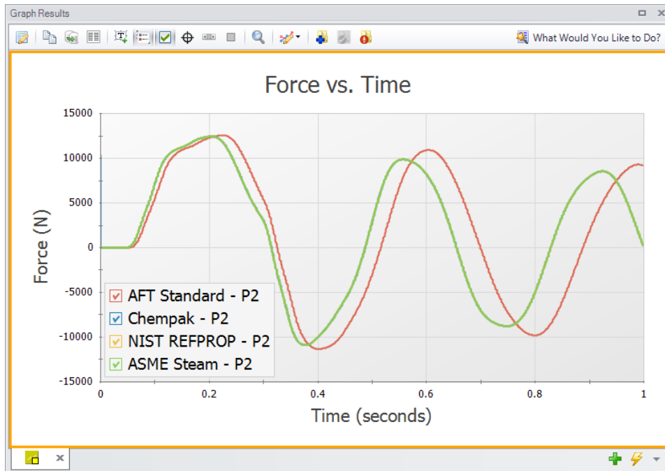
Figure 19: Effect of fluid property model on High Pressure Steam - Forces model. All runs use a Minimum Number of Sections Per Pipe of 1 and an Estimated Maximum Pipe Mach Number During Transient of 1.
