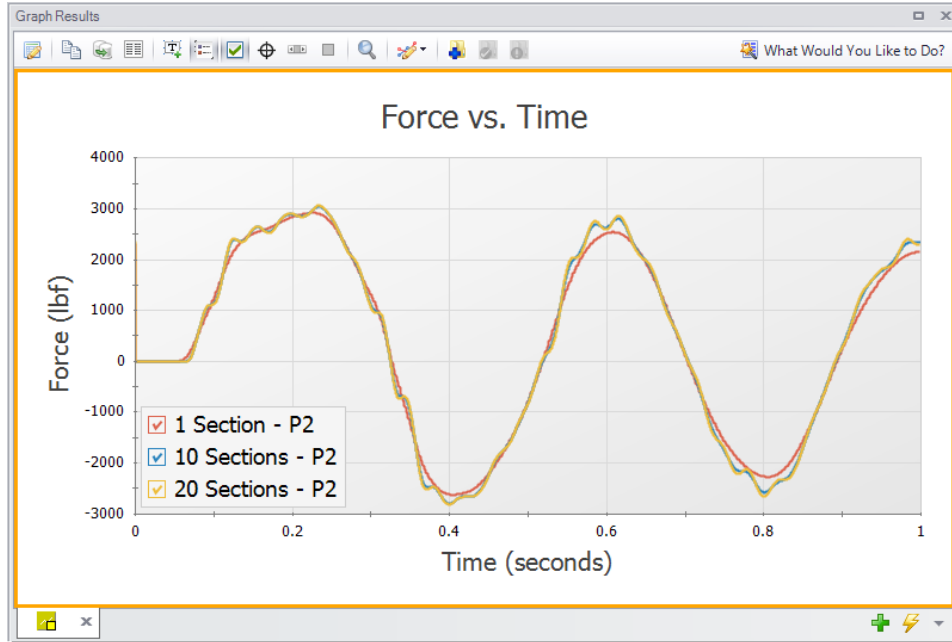
Figure 18: Effect of sectioning on High Pressure Steam - Forces model. All runs use the AFT Standard fluid library and a Maximum Pipe Mach Number During Transient of 1.
