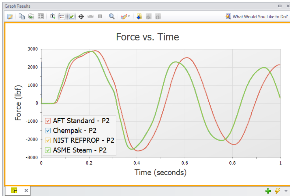
Figure 18: Effect of the fluid property model when all scenarios use a Minimum Number of Sections Per Pipe of 1 and an Estimated Maximum Pipe Mach Number During Transient of 1
