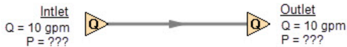
Figure 1: Model with two assigned flows. This model does not have a unique solution.
