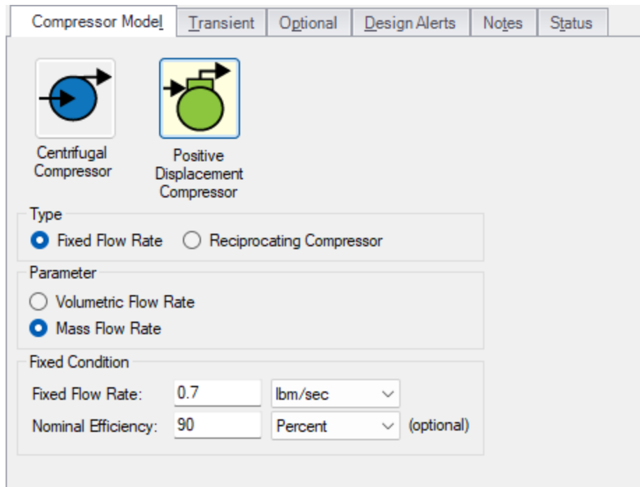
Figure 1: Fixed Flow Rate Positive Displacement Compressor model
