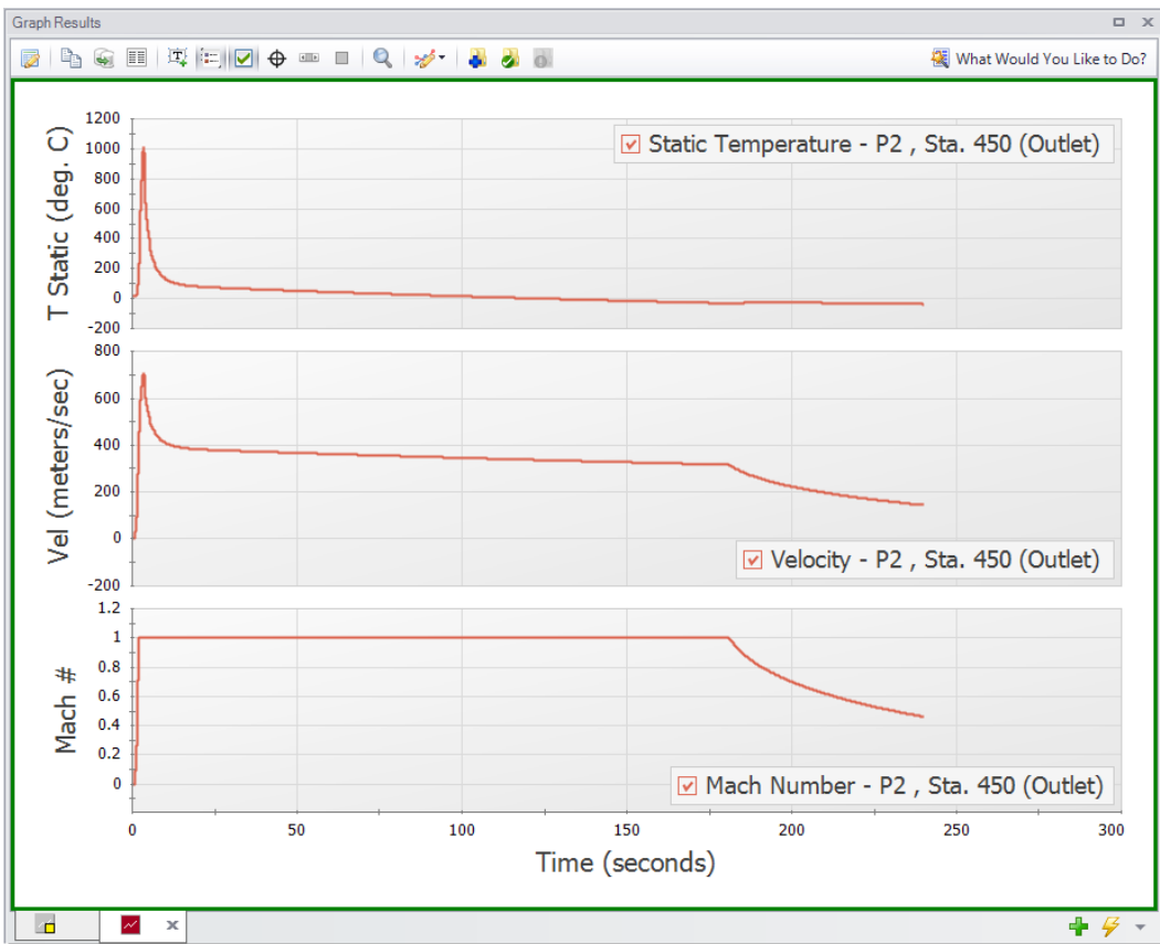
Figure 2.37 Temperature, velocity, and Mach number for the discharge of Pipe P2 with 6 sections minimum per pipe
