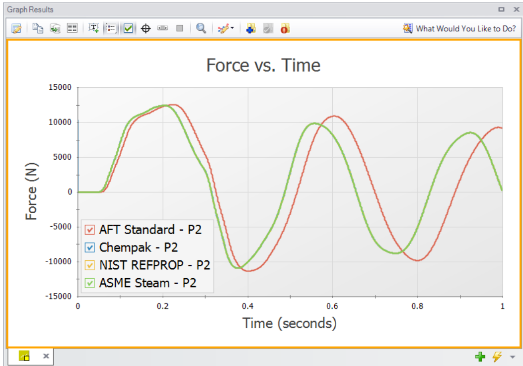
Figure 5.18 Effect of the fluid property model when all scenarios use a Minimum Number of Sections Per Pipe of 1 and an Estimated Maximum Pipe Mach Number During Transient of 1
